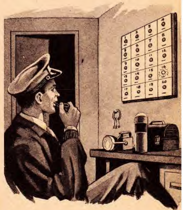
Trained dogs walk up and down the aisles of a department store at night (left). A guard watches the board in a separate room (right) where light bulbs light up as the dogs break the invisible light beams crossing the aisles.
